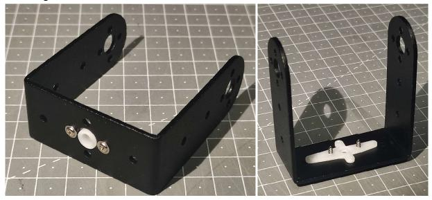
**Step 4:** Assemble the second servo cross lever to the U-bracket side using 2 long screws from the second servo bag
