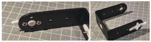
Step 5: Assemble both servos using the small screw from the servo bag
